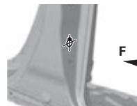
F4 Sliding Door Center Rail Mounting Hole \varnothing 6.3 (0.248)
