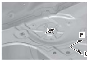
H4, h4 Floor Rear Extension A Locating Hole \varnothing 20 (0.79)
